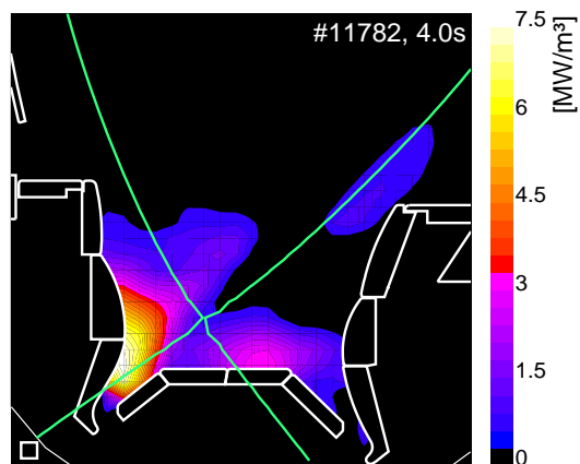
Fig. 3: Radiation profile for a shot with the outer strikepoint on roof baffle (horizontal target). The input power is 5MW.
