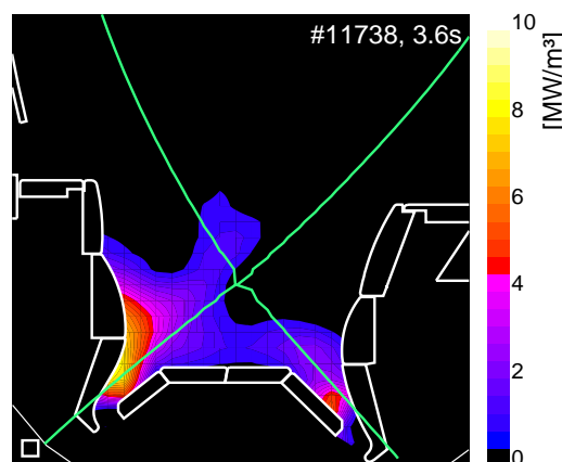
Fig 1: Reconstructed radiation pattern in the ASDEX Upgrade LYRA divertor with pronounced radiation peaks in the inner and outer divertor fan at the strikepoints. The input power is 5MW
