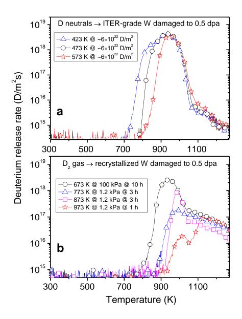
Figure 4. Thermal desorption spectra of  $D_2$  molecules for damaged ITER-grade W exposed to D neutrals (a) and recrystallized W exposed to  $D_2$  gas (b). Exposure temperatures, D implantation fluences, gas pressures and exposure durations are indicated in the legends. The TDS heating rate was 0.5 K/s. In both panels, the deuterium release rate is shown on a logarithmic scale.
