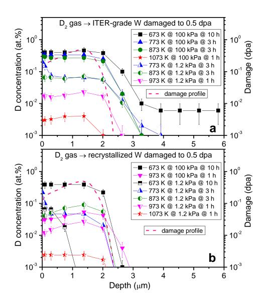
Figure 2. Depth profiles of deuterium retained in damaged ITER-grade W (a) and recrystallized W (b) after exposure to  $D_2$  gas. Exposure temperatures, gas pressures and exposure durations are indicated in the legends. In both panels, damage depth profiles as calculated by SRIM 2008.03 [16] are also shown.
