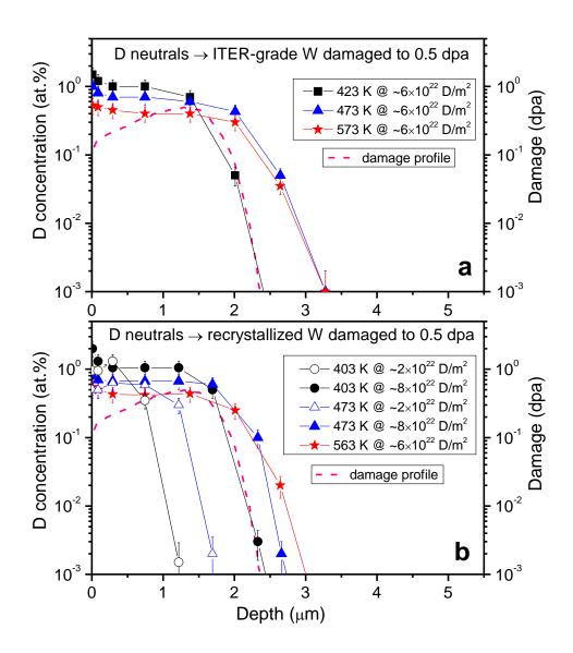
Figure 1. Depth profiles of deuterium retained in damaged ITER-grade W (a) and recrystallized W (b) after exposure to D neutrals. Exposure temperatures and D implantation fluences are indicated in the legends. In both panels, damage depth profiles as calculated by SRIM 2008.03 [16] are also shown.
