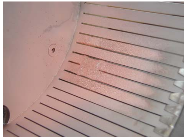
Figure 103: RADI Faraday screen with damaged fingers. The inner surfaces were covered previously with Mo.
