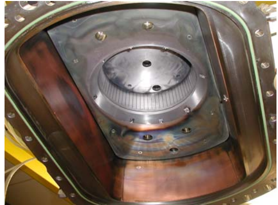
Figure 61: Mo coating of the Faraday shield and the source back plate including the cone
