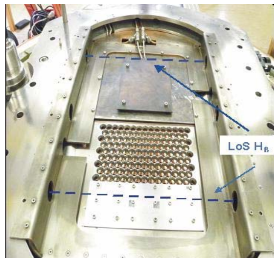
Figure 97. Partly covered plasma grid with the LOS of the H_\beta spectroscopy
