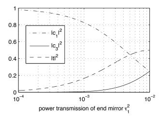
Fig. 4. Powers of the two reflected ports and the transmitting port as a function of end mirror transmittance  $\tau_1^2$  for a coupler with  $\rho_0^2 = 0.99$  and  $\eta_2 = \eta_{2,\text{min}}$  for a tuning of  $\phi = 0$ .
