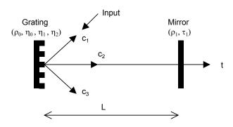
Fig. 2. A Fabry-Perot cavity with a 3-port grating coupler and a conventional end mirror. The amplitudes of the fields of interest  $(c_1, c_2, c_3, t)$  are indicated by arrows.
