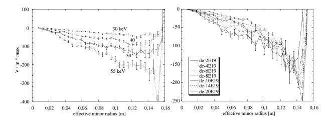
Fig.1: Calculations of radial profiles for  $\Delta E_r/\Delta t$  (r) in V/m msec. Left plot: variation of the injection energy (30 keV to 55 keV), right plot: variation of the electron density. Statistical error bars arising from the Monte Carlo procedure are given.
