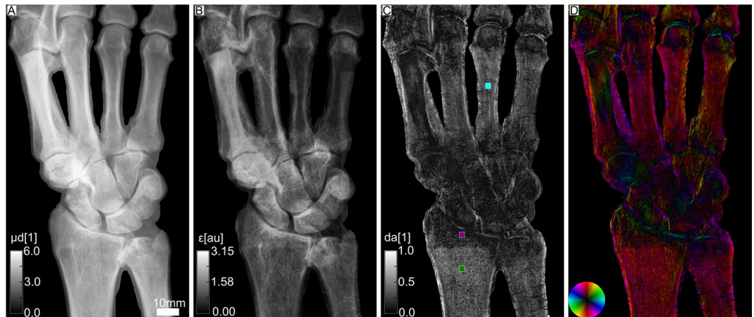
Figure 2. Attenuation and XVR images of a human hand, showing the radius, ulna, carpals and metacarpals. In (A) the integrated attenuation coefficient is depicted. (B) Depicts the mean scattering strength. (C) Illustrates the degree of anisotropy, i.e. the difference of maximum and minimum scattering divided by its sum. The mean values in the colored ROI's are da_{\text{cyan}} = 0.27 , da_{\text{purple}} = 0.08 and da_{\text{green}} = 0.41 . In (D) the orientation of scattering structures is color-coded according to the color wheel shown in the bottom left. Brightness once again corresponds to the degree of anisotropy.
