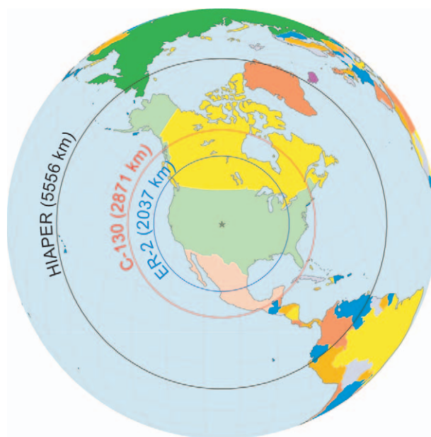
FIG. 3. A comparison of the maximum ranges for HIAPER (black circle), the NSF/NCAR C-130 (red circle), and the NASA ER-2 (blue circle). The circles shown represent the maximum distance to which each aircraft can fly from a base at Jefferson County Airport in Broomfield, CO (represented by the star), and return to the same base. The ranges shown correspond to flight of each aircraft at optimum altitude for ferry (12,500 m for HIAPER, 6100 m for the C-130, and 19,800 m for the ER-2) and with the maximum possible payload deployed on each aircraft.
