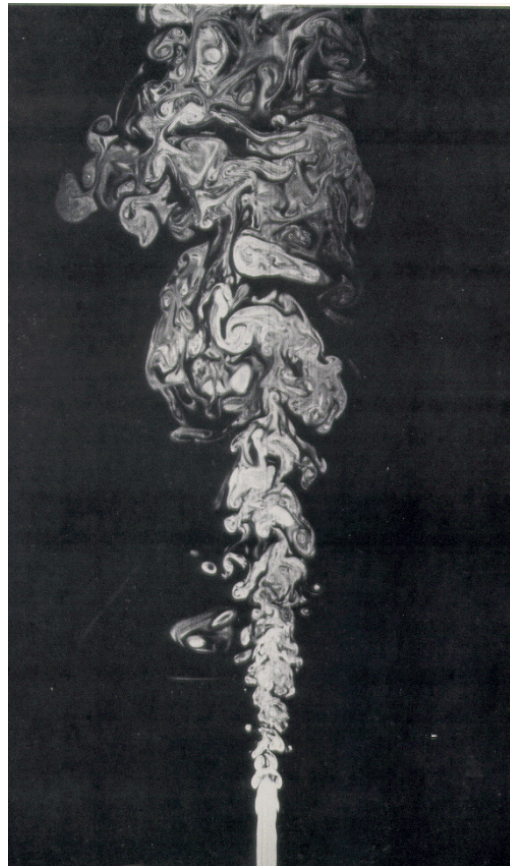
Figure 1.2: Snap-shot of a turbulent flow developing from an initial laminar jet flow. The formation of turbulent structures is apparent in the developed turbulence. (Picture from [VD82])
