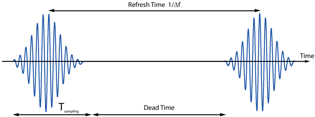
Figure 2.2: Two interferograms in time, separated by the refresh time 1/\Delta f . If information can only be gained in T_{\text{sampling}} a significant dead time is introduced between consecutive measurements.
