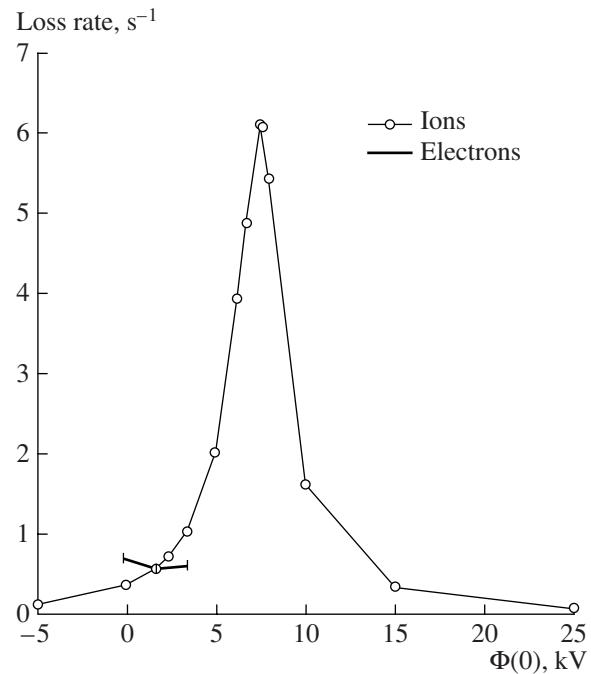
**Fig. 1.** Losses of monoenergetic 50-keV ions and electrons subjected to pitch-angle scattering with a normalized mean free path  $L^* = 3 \times 10^3$  ( $L^* = \lambda/L_c$ ,  $\lambda$  mean free path,  $L_c$  half the connection length) following the procedure of [9] versus the height of the electric potential applied in the quasi-isodynamic configuration of [6] with  $\langle \beta \rangle = 0.1$ , magnetic field strength  $B = 5$  T, and a plasma volume of  $10^3$  m<sup>3</sup>.
