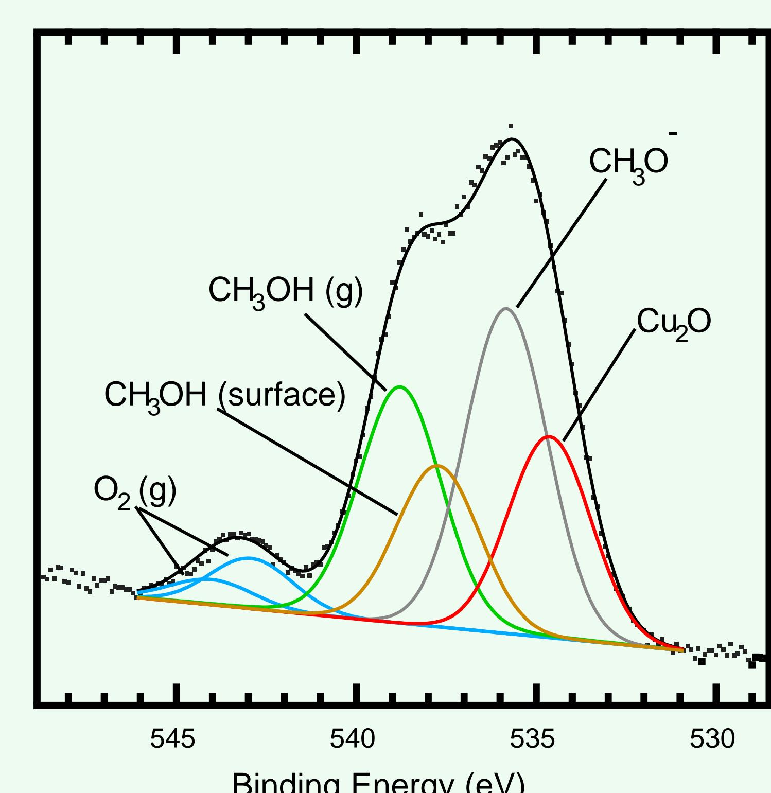
XPS O1s spectrum of a Cu foil in a gas mixture of 0.07 torr  $\text{O}_2$  + 0.34 torr  $\text{CH}_3\text{OH}$  @ 275 °C.
