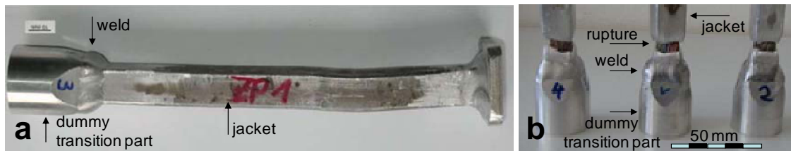
Figure 6: Test sample (a) and typical failure pattern of the axial pulling tests (b).
