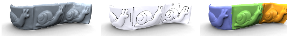
Figure 1.1: A 3D scan of a deformed plasticine sculpture with three snail figures. Our algorithm detects symmetries by looking at constellations of surface feature lines. This can be used for detecting deformable symmetries. Left: input data, middle: feature lines overlay, right: detected symmetries.
