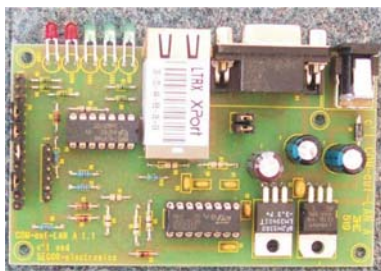
Figure 3: Lantronix's XPort provides a LAN-to-serial bridge and a web server
