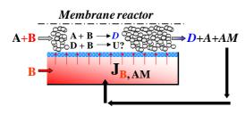
if the amount of A dosed through membrane additionally (AM) can be separated at the reactor outlet and fed again via a circular flow. For this background, the from the industrial point of view, interesting oxidative dehydrogenation of propane to propylene (limited intermediate) was analyzed. Therefore a reduced reactor model (isotherm, isobaric, plug flow) was utilized to evaluate the
