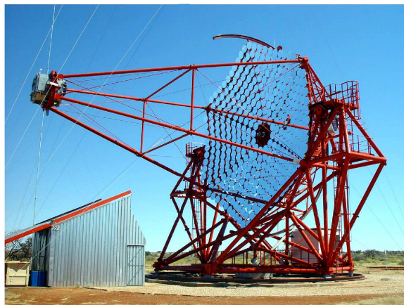
Fig. 2.7: One of the four Imaging Atmospheric Cherenkov Telescopes of H.E.S.S..
