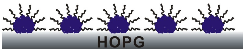
Figure 3.16. Model of ss-DNA- b -PPO hemimicelles (polymer in the core and DNA in the shell) adsorbed on HOPG surface. A monolayer with PPO adsorbed to HOPG and DNA facing to water formed firstly to provide template for the following hemimicelles formation.
