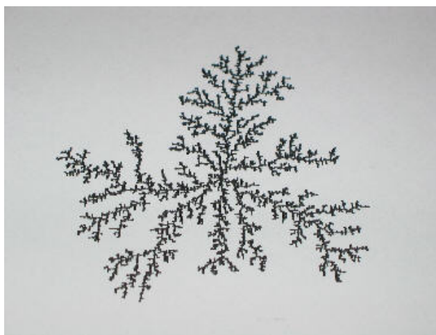
Figure 3.45. Witten-Sander cluster model grown on two dimensional square lattices which consists of 10000 particles.
