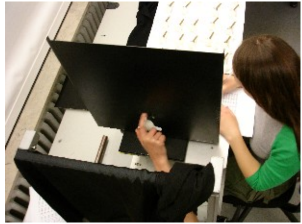
Figure 3: Experimental setup for haptic similarity ratings. The experimenter places the objects on a mount placed behind an opaque curtain. The participant haptically explores the object using one of four exploratory procedures.
