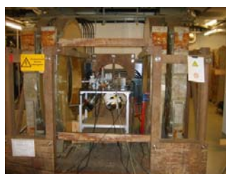
Figure 6: Helmholtz coil set-up with W7-A coils for testing an ACORD-24 analyser in an outer magnetic field
