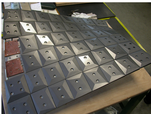
Fig. 4. Heat shield with clamped graphite tiles, two tiles on the left inside are removed to view CuCrZr plates of the 3D-shaped cooling structure. Every tile is differently machined with facets according to physics specification. Screws are made of TZM.
