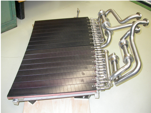
Fig. 2: Full scale prototype HHF target module with dummy target elements. The target elements are water-cooled in parallel from stainless steel manifolds. The inlet/outlet connections to the feeding ports are also shown.
