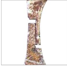
Fig.11 Crosssection of the new labyrinth sealing between cooling channels.
