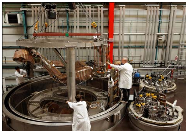
Fig.1 Mounting of a non-planar coil into the cryostat
