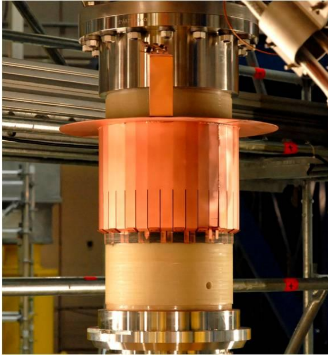
Figure 7. Cryo leg without the bellow and the bearings
