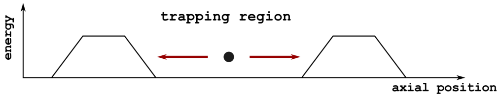
Figure 2.10: Simplified drawing of the axial electric potential, which is applied on the mirror electrodes of the multi-reflection time-of-flight device to create a trapping region.
