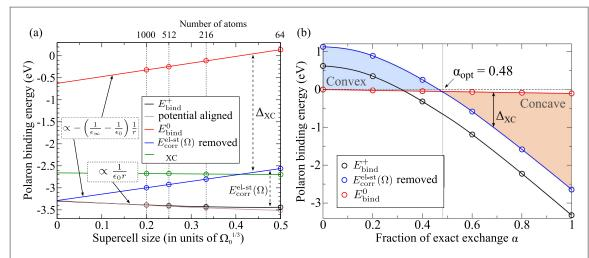
**Figure 2.** (a) Supercell dependence of the polaron binding energy and exchange-correlation error for HSE( $\alpha=1$ ). The atomic positions are fully relaxed for each supercell size by optimizing the geometry of the charged cell. (b) Dependence of the polaron binding energies on the fraction of exact exchange. The fixed geometry of the  $3\times3\times3$  supercell from figure 1, panel (a) is used and binding energies for different fraction of exact exchange are calculated.
