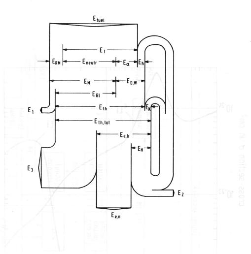
Fig. 4 Detailed energy flow chart of a fusion power plant
