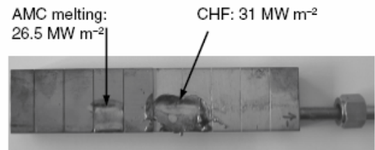
Figure 2. View of a target element surface with removed CFC tiles. 26.5\text{ MW/m}^2 loading resulted in the partial melting of the AMC surface. For 31\text{ MW/m}^2 loading CHF and burn out occurred.
