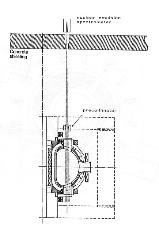
Fig. 5: Arrangement of precollimator and nuclear emulsion spectrometer at JET,
