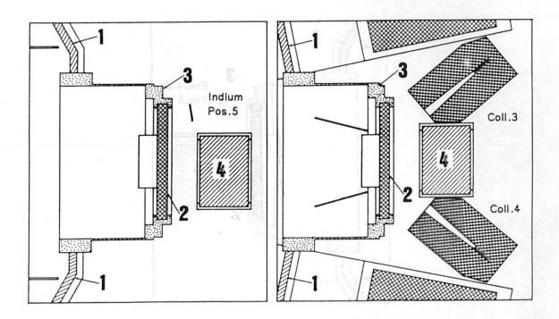
Fig. 6: a) Vertical cross-section through the quartz window and indium sample at position 5
