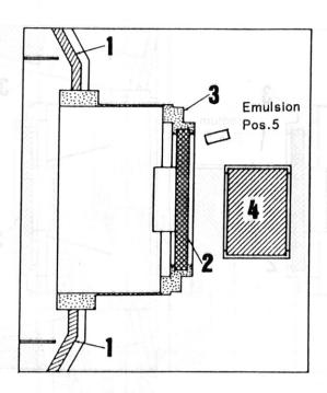
Fig. 7: Vertical cross-section through the quartz window and nuclear emulsion box at position 5
