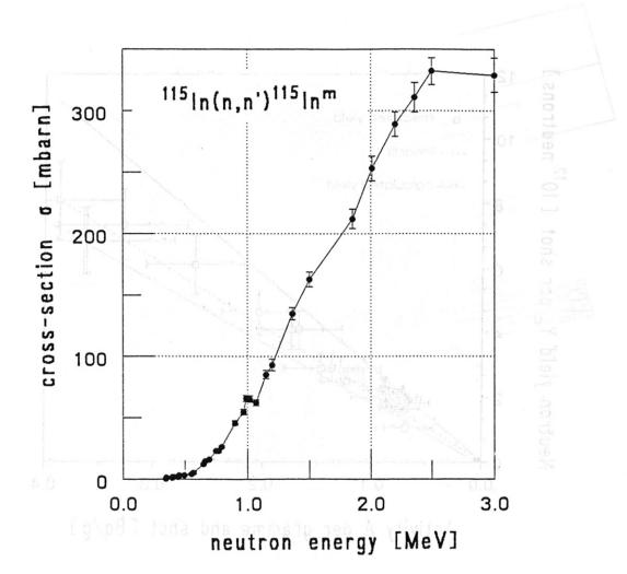
Fig. 2: Cross-section for indium activation [4]
