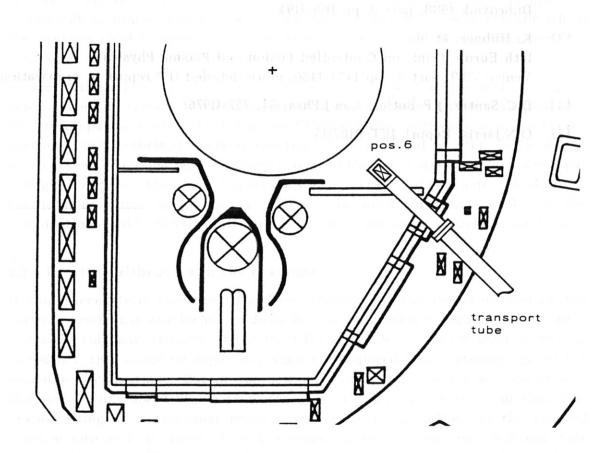
Fig. 1: New position 6 at ASDEX inside the vessel for indium activation and nuclear emulsion measurements
