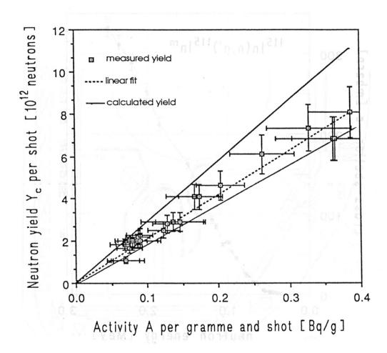
Fig. 3: Neutron yield  $Y_c$  from counters as a function of sample activity A
