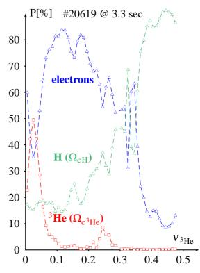
Figure 3: rf power distribution in a H(<sup>3</sup>He) plasma as function of <sup>3</sup>He concentration.
