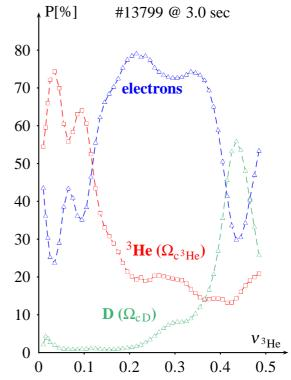
Figure 2: rf power distribution in a  $D({}^{3}He)$  plasma as function of  ${}^{3}He$  concentration.
