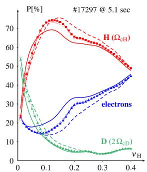
Figure 1: rf power distribution in a D(H) plasma as function of the H concentration for  $n_{\varphi} = 12$ : solid lines with Maxwellian distribution functions (df) for the minority, open symbols with df calculated by SSF-PQL with 4 MW of coupled power, and full symbols are the second iteration of TORIC-SSFPQL. The dashed lines are the first iter. with 10 MW of rf power.
