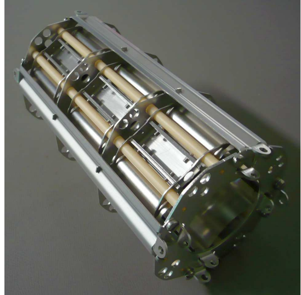
Fig. 3.3: Einzel lens consisting of three segments in longitudinal direction which in turn are subdivided into four electrodes. Latter form a set of three quadrupoles.
