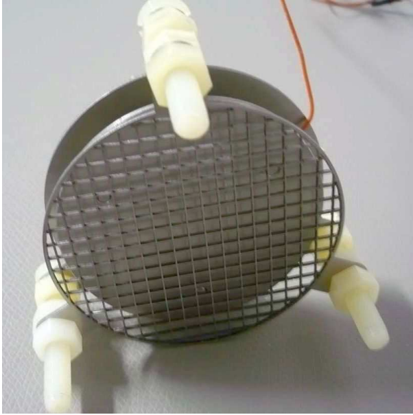
Fig. 3.7: Faraday cup with a metal grid attached to it. The grid can be used to reflect emitted secondary electrons and reduces induced signals from switching the endcaps of the Penning trap. Polyamide screws (ivory-coloured) are used to insulate the cup from the holder (not shown). Taken from [UD11]
