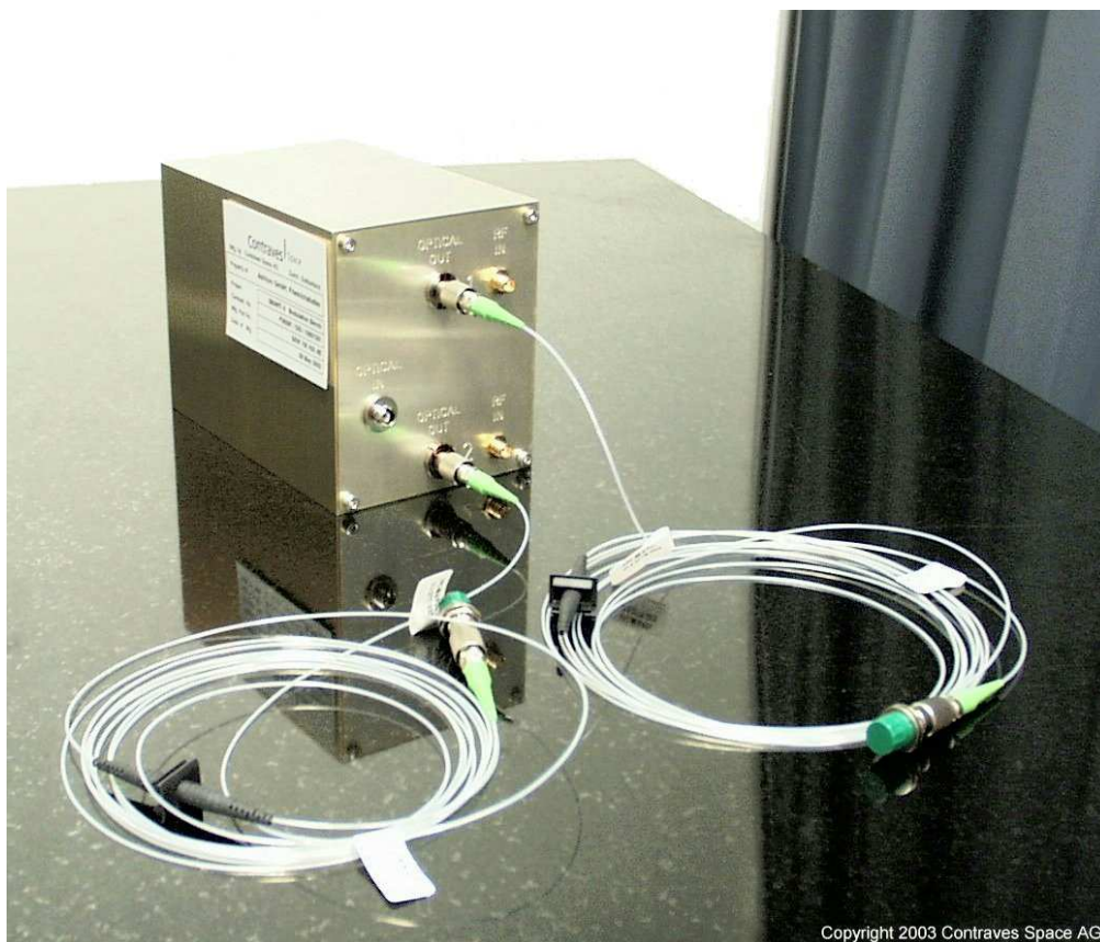
Figure 2.12: Prototype for a space qualifiable modulation bench developed by Contraves
