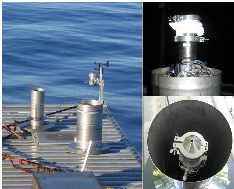
Figure 5.1: The inlet system on top of the sea-container. The smaller one in the back is the inlet for \text{H}_2\text{SO}_4 measurements while the bigger one in the front is the one for \text{SO}_2 measurements. On the top right side the setup for background measurement with the filter paper is shown. On the bottom right side the inlet icon cone in the center of the protection pipes is shown.
