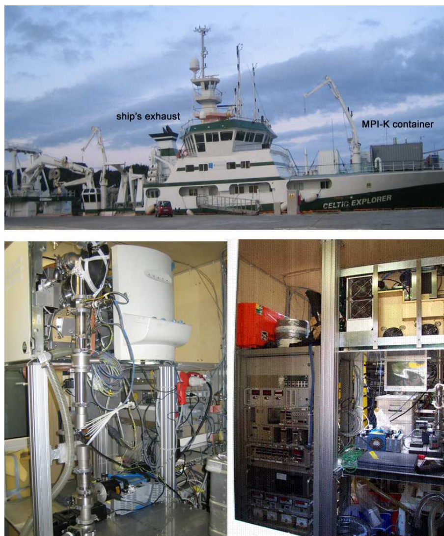
Figure A.21: Above: The Celtic Explorer in the harbor of Killybegs, North of Ireland. The MPI-K container is placed on the front deck while the exhaust is on the after deck. Below: Photograph of the IT-CIMS application inside the 20 feet sea-container; the right photograph shows the rack with supporting components, the left photograph shows the front of the spectrometer and the exhaust tube.
