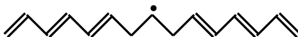
Figure 2.9: The free-radical defect (soliton) in trans -polyacetylene chains with odd numbers of carbon atoms.
