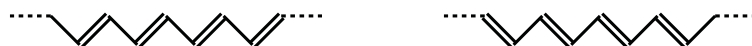
Figure 2.8: The two degenerate ground state patterns of in an ideal quasi 1D trans -polyacetylene chain.
