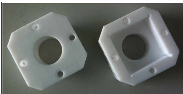
Figure 2.6 Image of two parts of a PTFE trough for the horizontal deposition of colloidal particles. A cleaned glass slide is placed in the bottom part (right) and the top part (left) is put on top and fixed with four screws.
