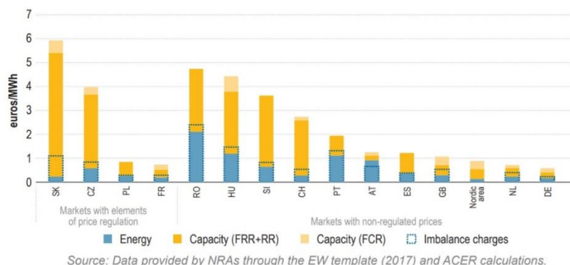
Figure 45: Overall costs of balancing (capacity and energy) and imbalance prices over national electricity demand in a selection of European markets in 2016 (ACER and CEER, 2017) 104
