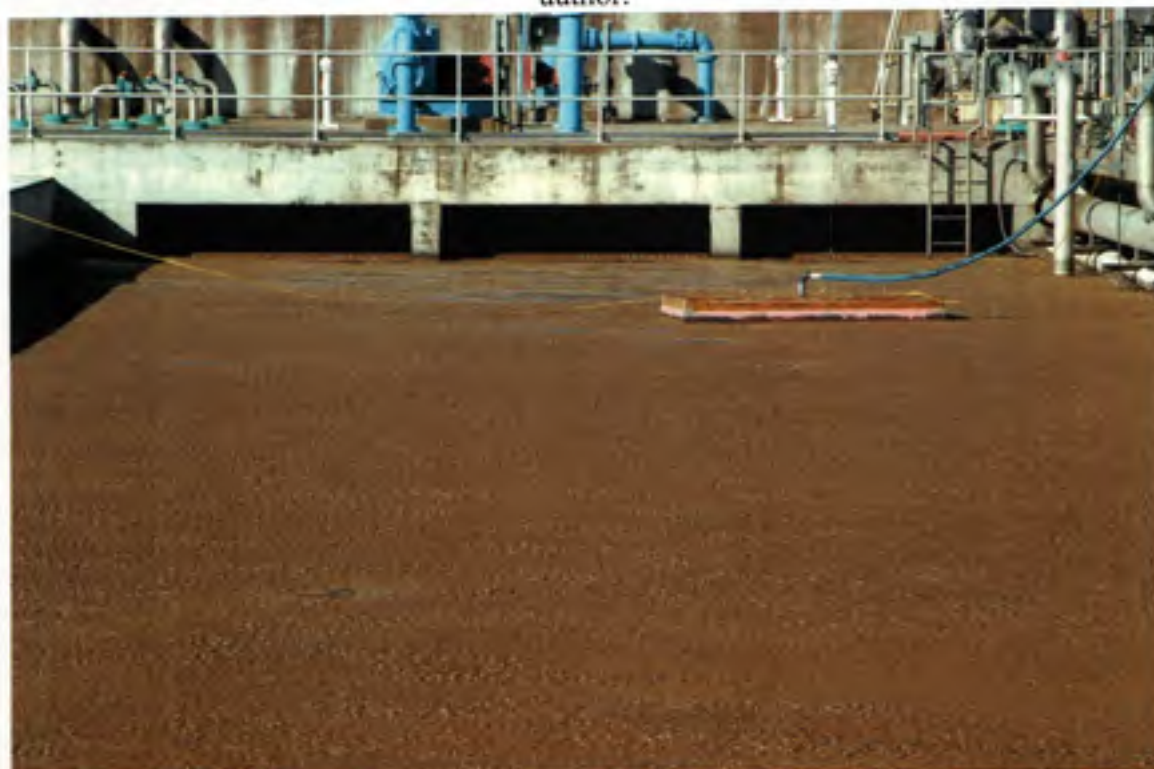
Photograph 2. Off-gas hood floating on the ASP Tank 11 during testing (January). Photograph taken by the author.
