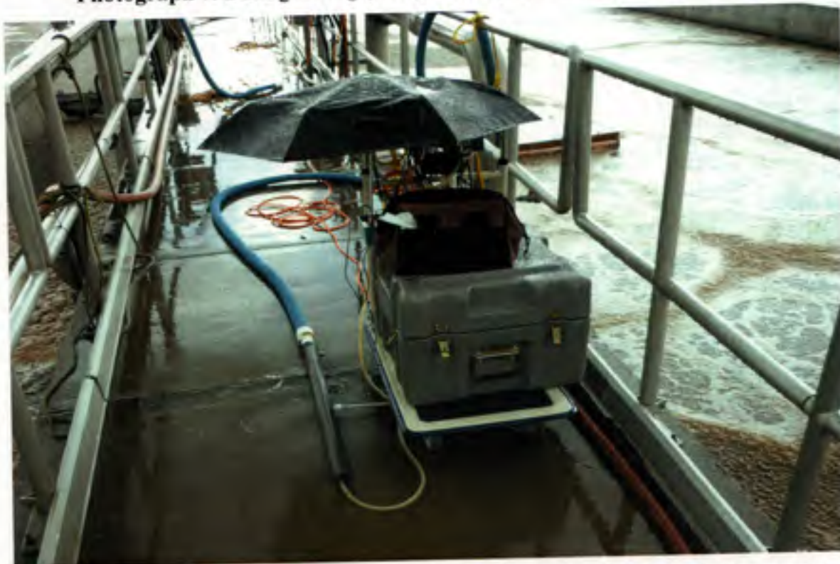
Photograph 8. Dr. Rosso's off-gas analyzer during the testing. Photograph taken by Diego Rosso.
