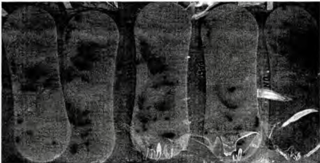
Figure 14. Pasteurization and filtration experiment. Qualitative comparison of dried LTB pads with various waters spiked with E. coli B (target 5 CFU/mL). (Left to right) University Lake water, pasteurized and filtered sewage spike, filtered sewage spike, pasteurized sewage spike, and untreated sewage spike (10 CFU/mL total E. coli ).
