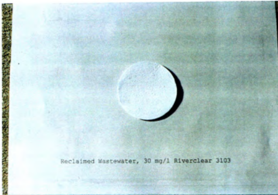
Figure 5-4c Fabric Staining Potential of Reclaimed Wastewater with Coagulation (30 mg/l Riverclear 3103).
