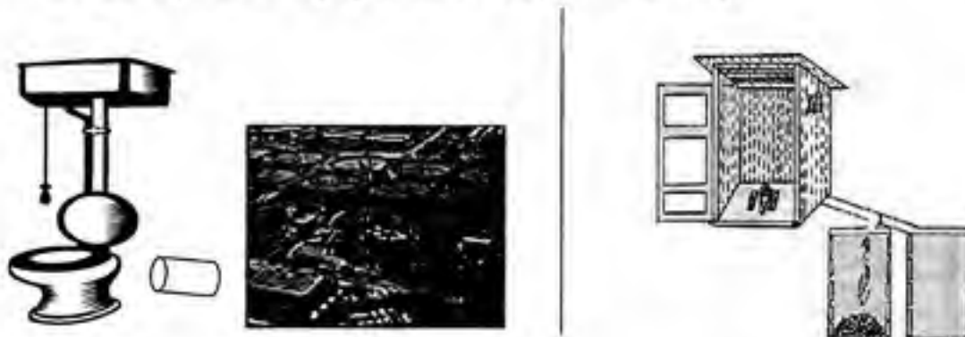
Figure 1.1 – Schematics of the "Flush-Discharge" and "Drop-Store" systems
