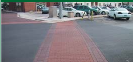
Textured pavement creates a threshold that signals an entrance to drivers. 3
