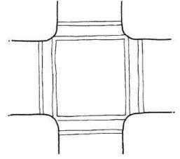
According to the Manual of Uniform Traffic Control Devices (MUTCD), the solid white lines must be at least 6 inches thick, mark both edges of the crosswalk and be spaced at least 72 inches apart. The ladder design is the most visible type of pedestrian crosswalk marking for motorists.
