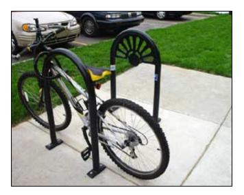
Below are two outdated bicycle racks, unsuitable for most modern bicycles. Both can cause damage to front wheels, and bicycles often do not fit in either model.
