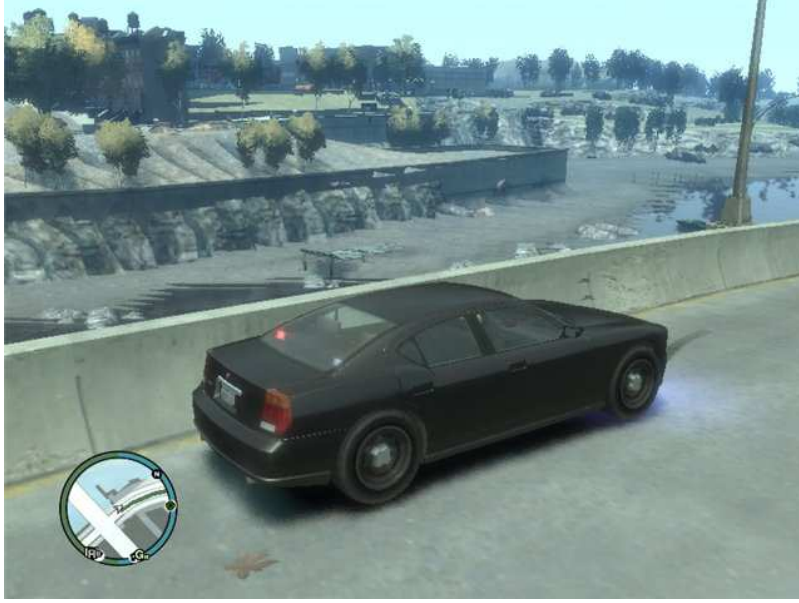
Figure 2.3: Z-fighting in the shoreline of a frame from “Grand Theft Auto: IV.”
