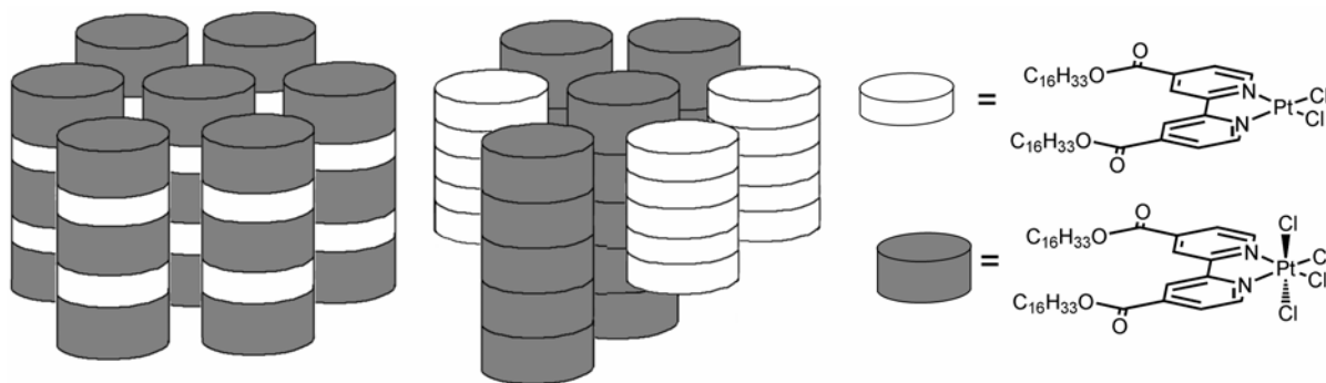
Figure 4-11. Possible methods of formation for a \text{Col}_H mesophase of 1:1 \text{PtL}^{16}\text{Cl}_2/\text{PtL}^{16}\text{Cl}_4 ; MX chain interactions within [\text{PtL}^{16}\text{Cl}_2\text{-PtL}^{16}\text{Cl}_4]_m columns (left), and random distribution of individual [\text{PtL}^{16}\text{Cl}_2]_m and [\text{PtL}^{16}\text{Cl}_4]_m columns (center).
