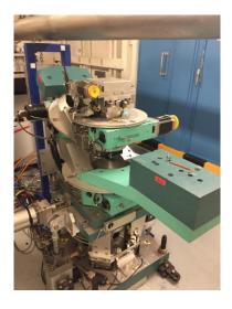
Figure 1.3 A photo of the sample positioning stage in the MRT experiment room at ESRF Biomedical Beamline ID17
