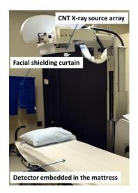
Figure 2.8 The s-DCT prototype installed at the Cystic Fibrosis and Pulmonary Diseases Research and Treatment Center, at UNC Marsico Lung Institute for clinical trials
