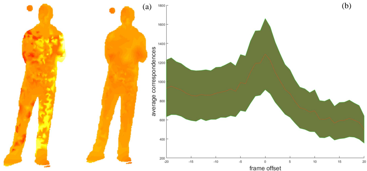
Figure 4.7: (a) show depth map generated from raw correspondences (Left) and the corrected correspondences (Right). (b) Average correspondences with different offsets (red curve), the green boundary should be the plus minus standard deviation.
