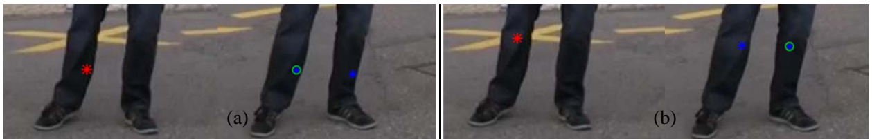
Figure 4.4: Red stars: Feature point in reference frame. Blue stars: Matched feature points in the target frame. Green circles: Points with highest NCC values. In (a), the point with the highest NCC value is actually the correct correspondence. However, in (b), the green circle is indicating the wrong match. The other candidate is the correct correspondence and should be used for triangulation.
