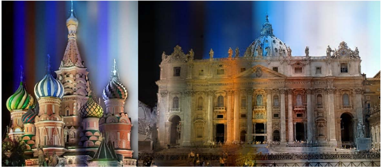
Figure 5.9: Failed cases for our method. Artifacts appear mainly on the domes and round facades which deviate from planar surfaces.
