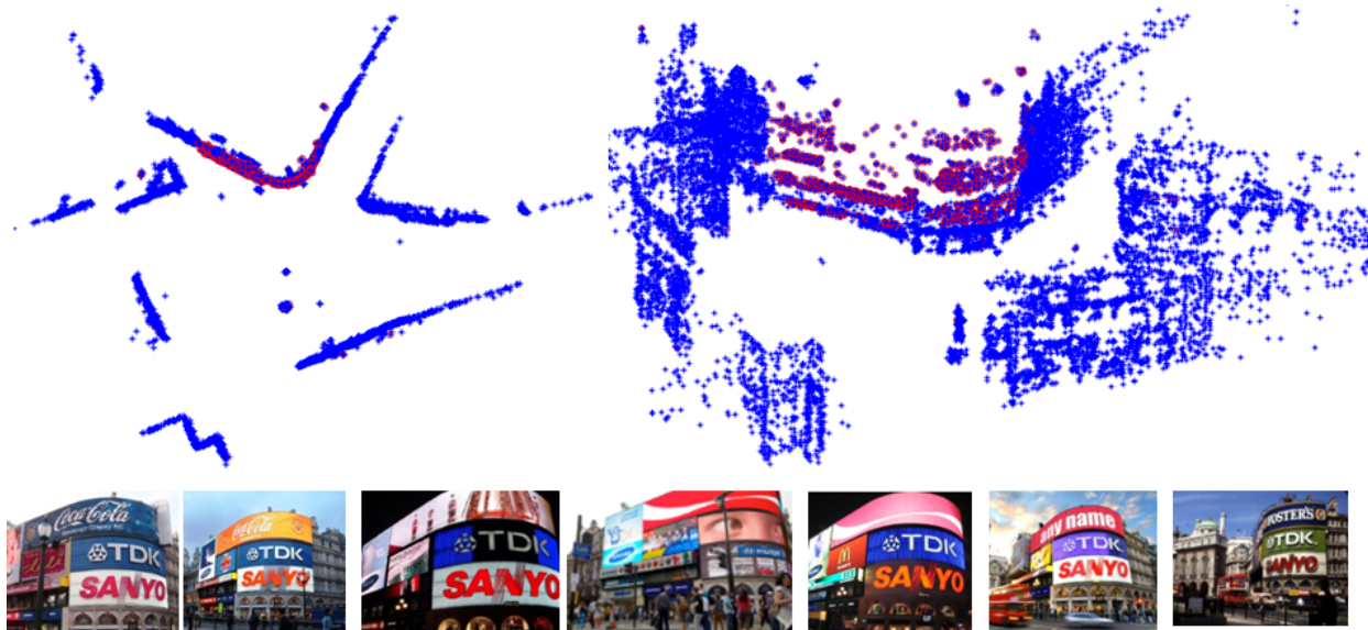
Figure 3.6: Identification of dynamic textures within existing SfM estimates. Top Row: birds-eye and frontal view of estimated sparse structure for Piccadilly Circus. Blue dots are 3D features with persistent color across the dataset. Red dots are 3D features determined to have sporadic color. The bottom row shows sample images in the dataset. We associate color persistence with predominantly linear variation in the RGB space.
