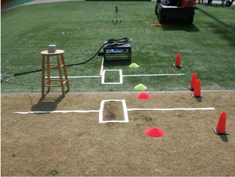
Figure 1. Transmitter placed between two playing surfaces to establish global reference frame of the system.
