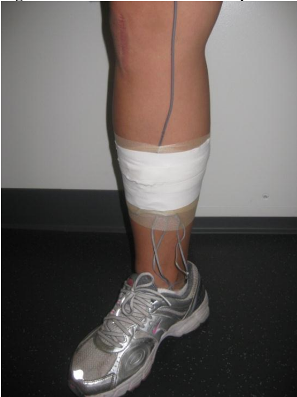
Figure 4. The attachment of the 4 pressure sensors' connection wires to the leg.
