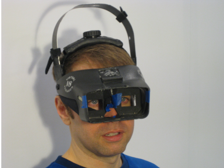
Figure 4.2: The modified V8 HMD ,with display elements removed so that subjects could see through the casing to the world-fixed display. Note the Hiball tracker is not shown in this picture but was mounted on top of the device during experimentation.
