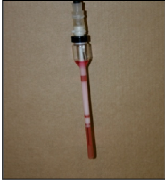
Figure 2-8: The final fluidized-bed design with just a top baffle and percolating beads.
