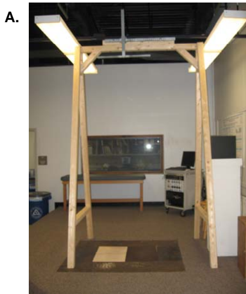
Figure 3. Adjustable drop bar used to complete 0.60 m double leg drop landings (A) and depiction of biofeedback display with knee flexion angle target window and cursor indicating instantaneous knee flexion angle (B).
