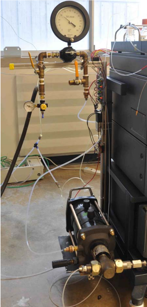
Figure 4-6. A photograph of the pneumatics sub-system showing mounting locations. Note the ball valves for manual shut-off and release of gas pressure to the -903. These are installed as a safety mechanism in case rapid decompression is required without the use of the computer controls.
