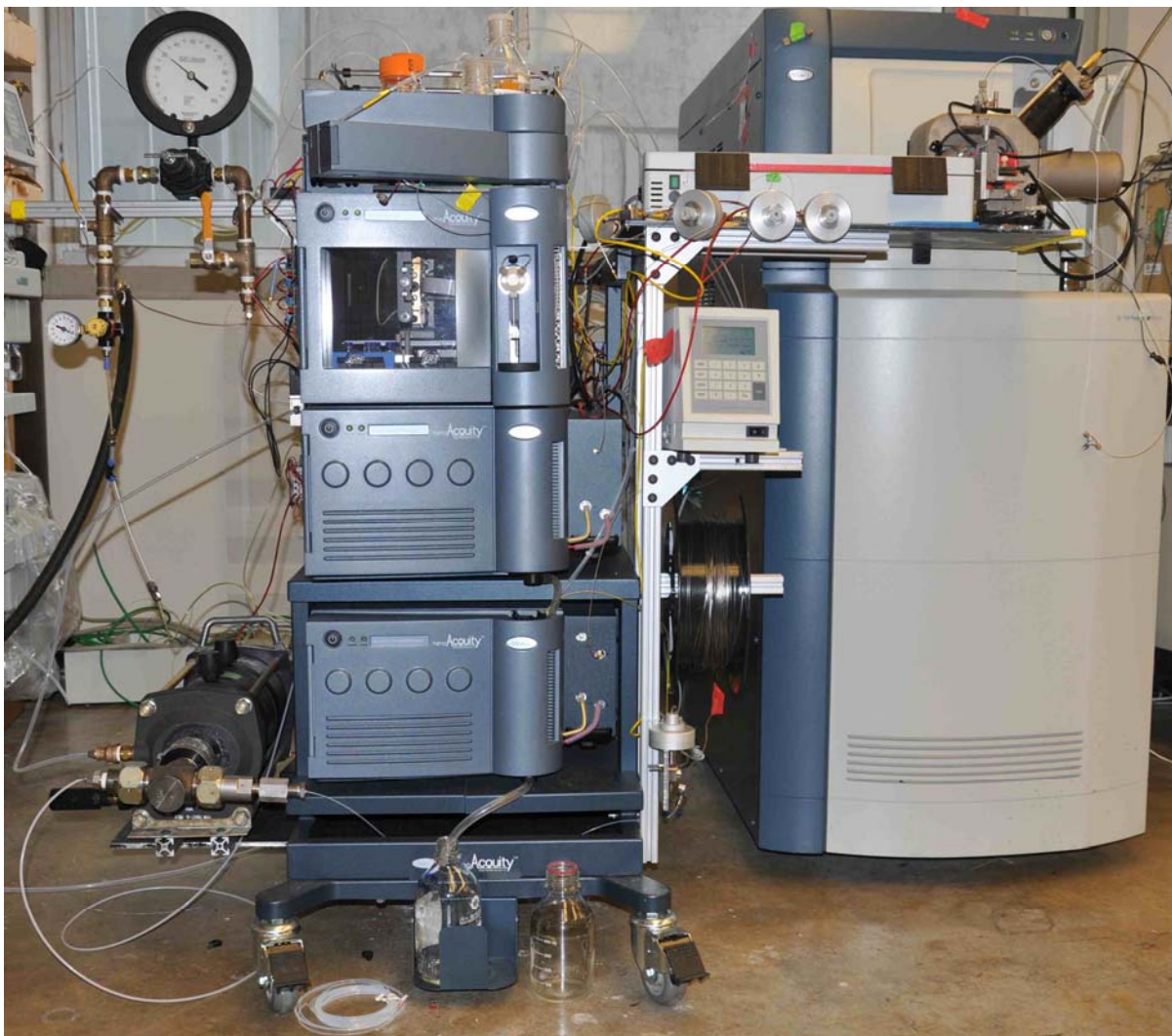
Figure 4-4. The nanoAcquity UPLC with the XUPLC modification installed. Pneumatic components are primarily located on the left side of the nanoAcquity stack with the exception of the Valco on/off valves. The column heater is mounted to position the outlet of the capillary column near the mass spectrometer source. A gradient storage loop is wound around a spool and mounted below the temperature control module on the lower right of the nanoAcquity.
