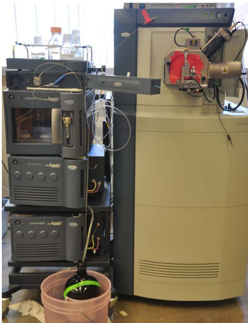
Figure 4-3. A Waters nanoAcquity UPLC with detection by a Waters QTOF-Premier mass spectrometer. The pressure limit of the nanoAcquity is 10,000 psi.
